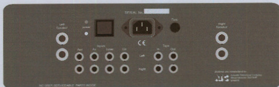
Diagram 1 - SIA2-150 rear panel and connectors
